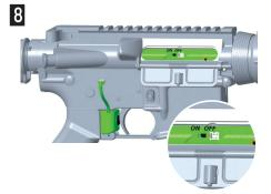
Connect the trigger switch cable with the Flash Bolt and switch main switch to "ON".
